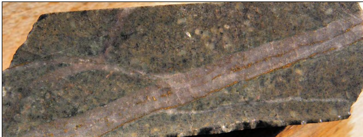
Figure 7-9 Photo of a classic B-style quartz vein with a chalcopyrite-filled centre-line cutting an irregular, wormy A-style quartz vein (Whistler Deposit, WH 08-08, ~123.0m)
