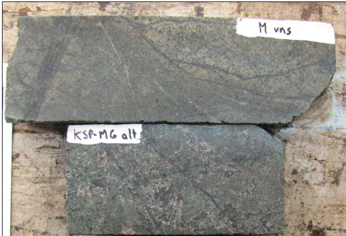
Figure 7-8 Photo of irregular M-veins in dark magnetite alteration of mafics (upper) and pervasive pink-black blotchy k-feldspar and magnetite alteration (lower) with wormy quartz + magnetite + chalcopyrite A-veins (Whistler Deposit)
