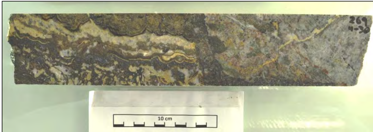
Figure 7-12 Photo of quartz-carbonate vein from Raintree West (WH11-030) showing well-developed colliform banding and coarse-grained sphalerite and galena
