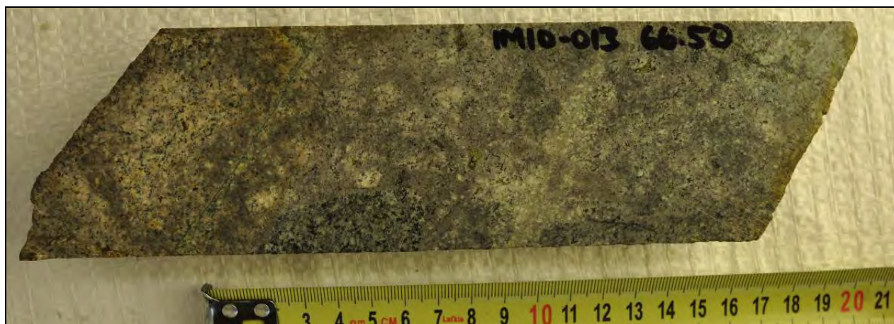
Figure 7-24 Photo of monzonite-matrix intrusive breccia with patchy albite alteration, silicification and disseminated chalcopyrite
