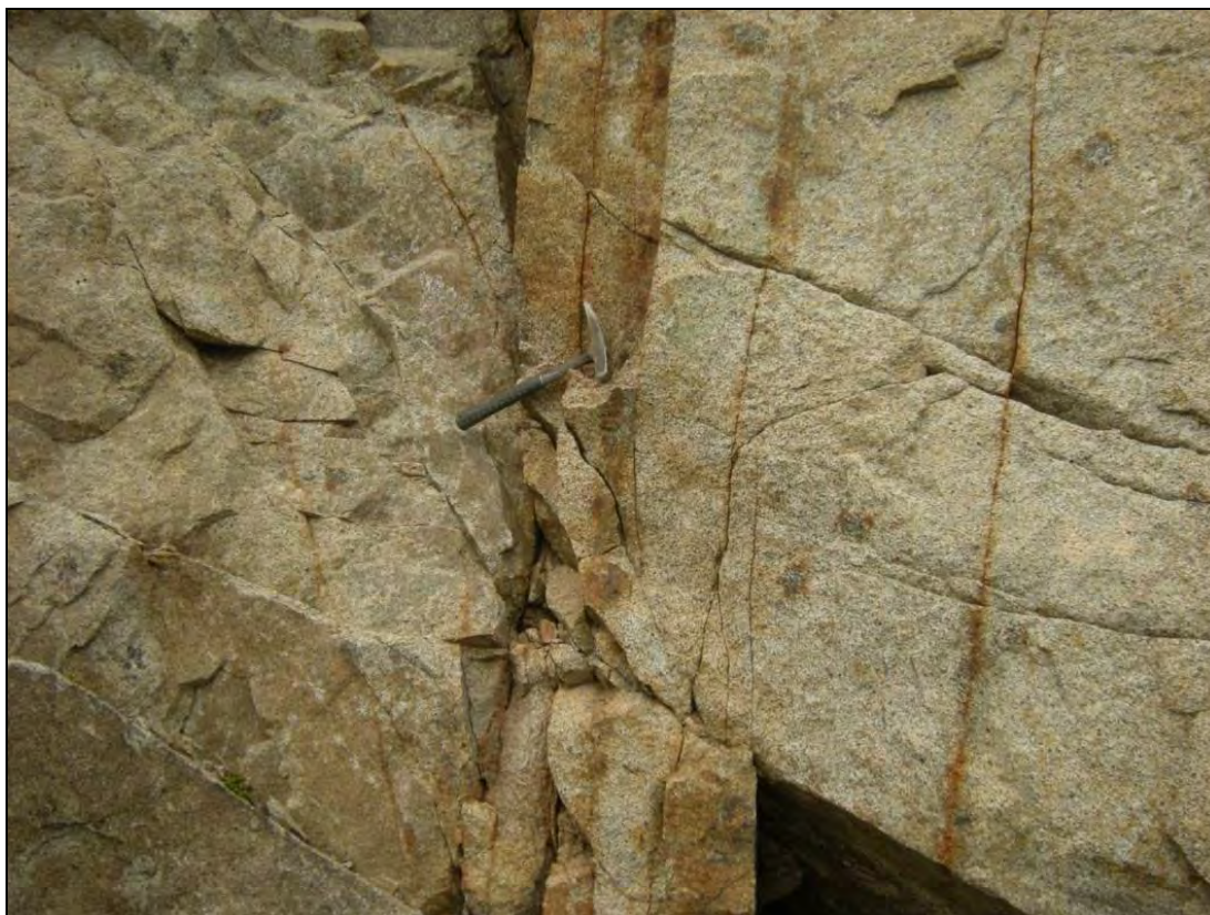
Figure 7-27 Detail view of Biotite Monzonite Northwest of Muddy Creek, cut by sub-vertical limonite-stained fracture fillings of chalcopyrite-arsenopyrite (~1-3 per metre).
