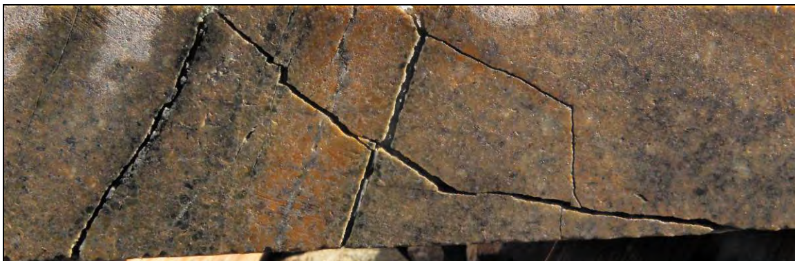
Figure 7-20 Whistler, WH 08-08, partially leached gypsum-filled fractures.
