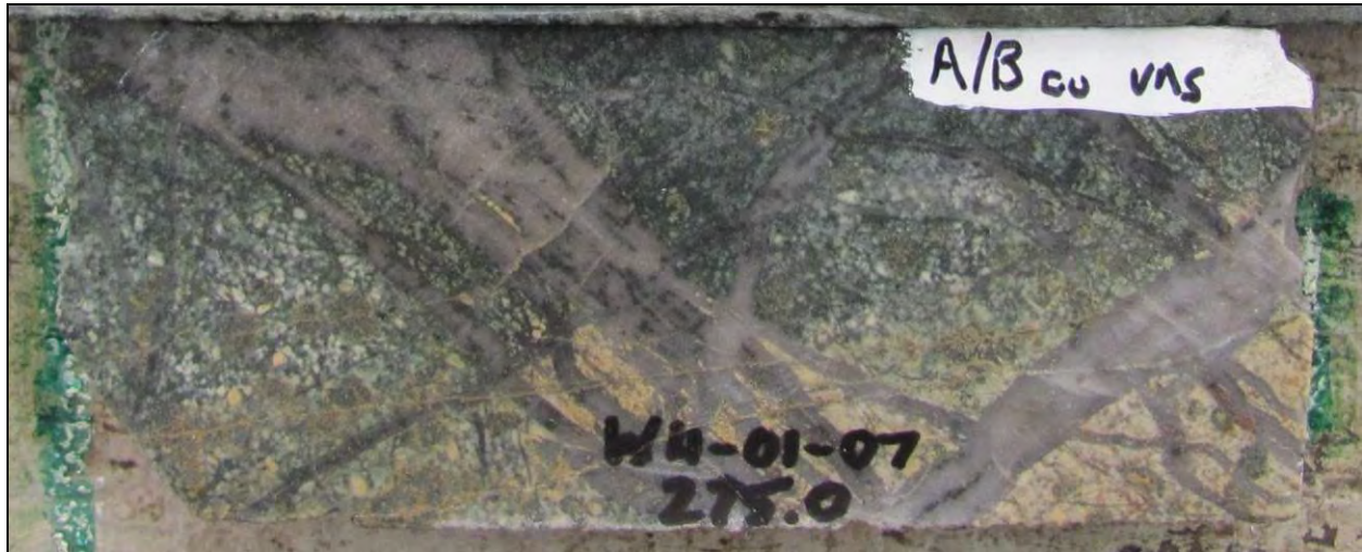
Figure 7-10 Photo of chlorite-sericite (+calcite) alteration overprinting potassic – magnetite alteration in a zone of quartz vein stockwork, subsequently cut by later Dpy veinlets with sericitic and iron-carbonate halos (Whistler Deposit)
