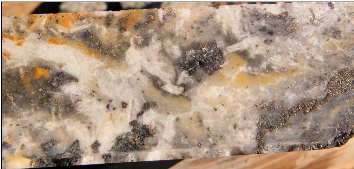
Figure 7-19 Whistler, WH 08-08, Late Quartz-calcite Vein with Galena and Sphalerite.
