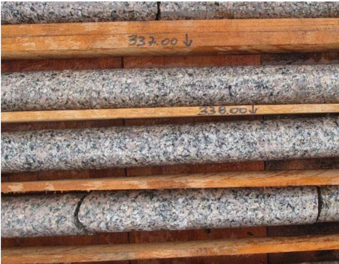
Figure 7.4 - Example of fresh, un-altered monzogranite
