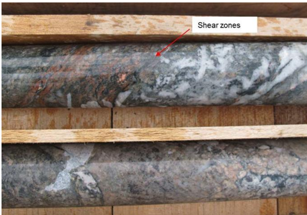
Figure 7.10 - Examples of shear zones containing quartz veins in drill core
