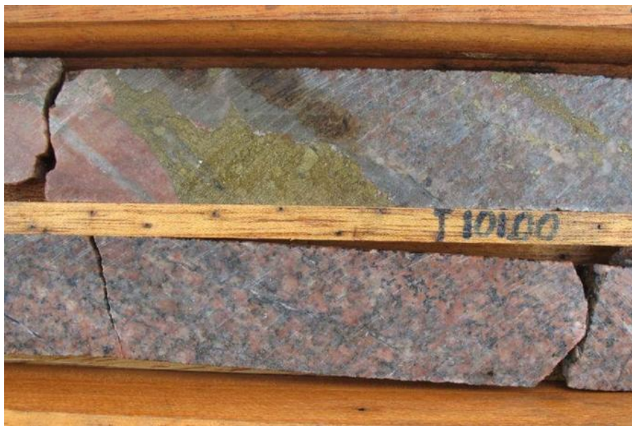
Figure 7.14 - Example of semi-massive, veinlet, and disseminated pyrite mineralization
