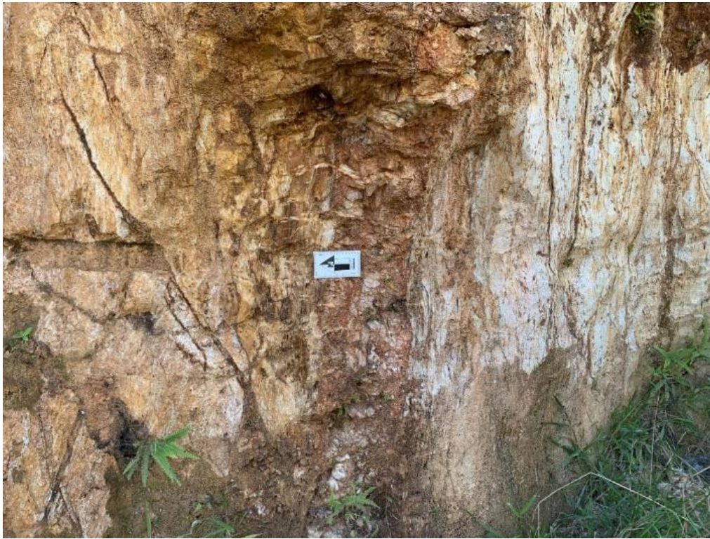
Figure 7.11 - Example of shear zone in saprolite containing sulphide veinlets. View looking east
