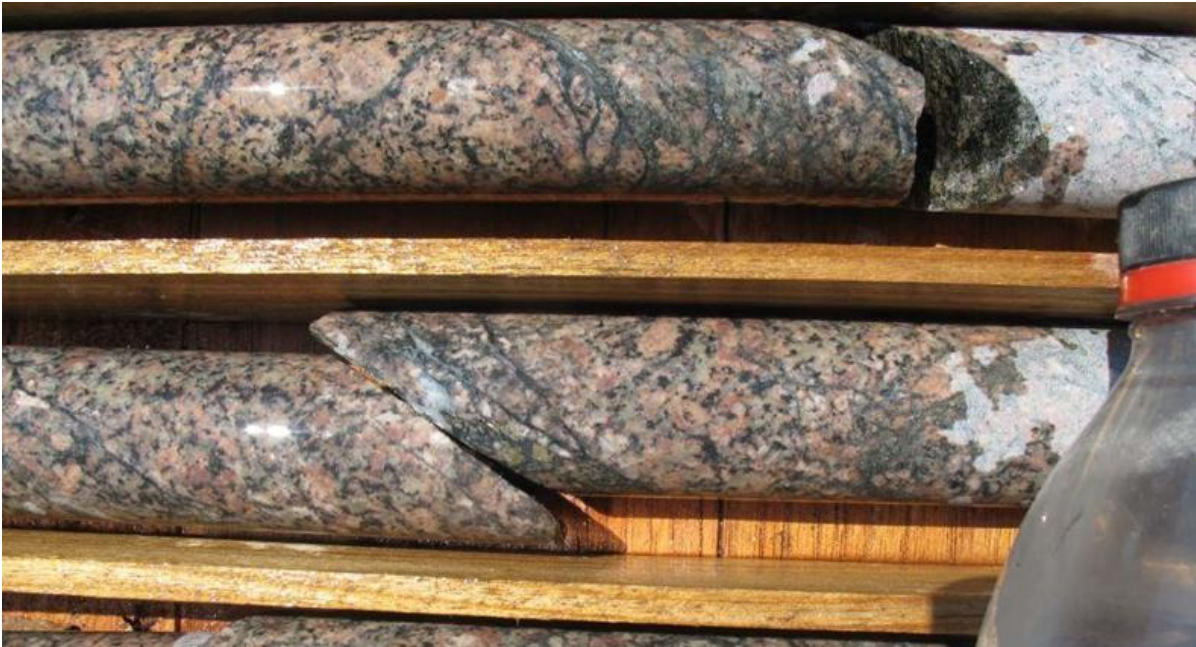
Figure 7.6 - Example of K-Feldspar-Epidote-Chlorite Alteration
