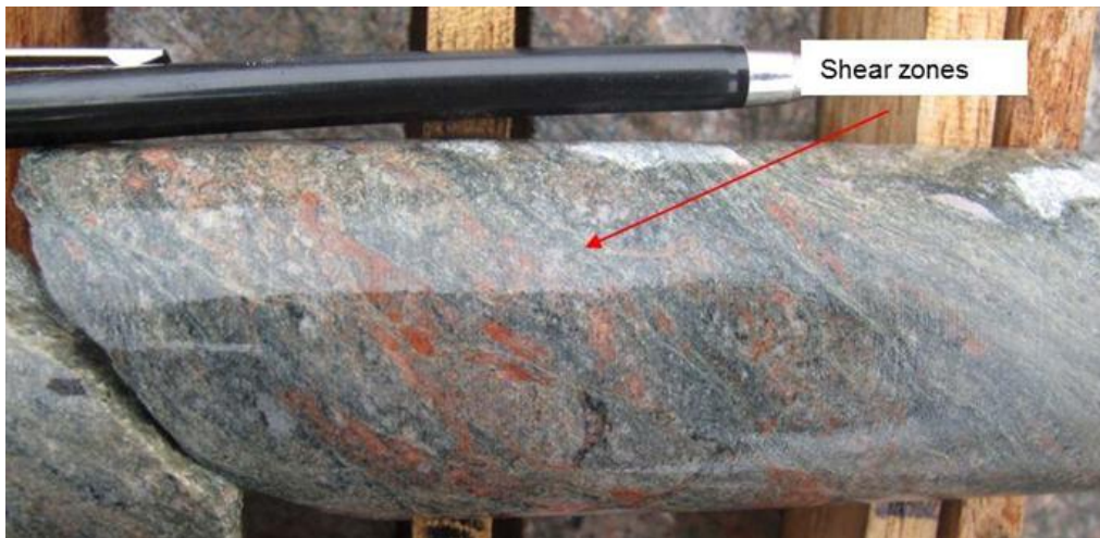
Figure 7.9 - Example of a small scale shear zone in drill core
