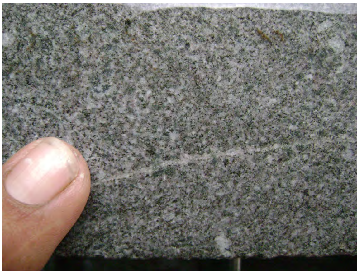
Figure 7-6 LMDDH-008-288m. C1 Porphyry with Pervasive Biotite-Magnetite Alteration of the Matrix and Actinolite Alteration of Primary Magmatic Mafic Phenocrysts
