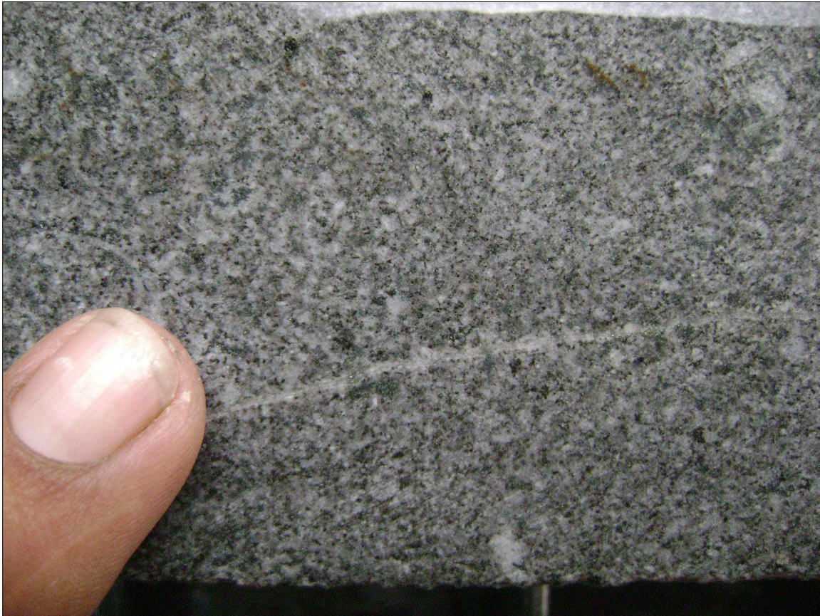
Figure 7-6 LMDDH-008-288m. C1 Porphyry with Pervasive Biotite-Magnetite Alteration of the Matrix and Actinolite Alteration of Primary Magmatic Mafic Phenocrysts
