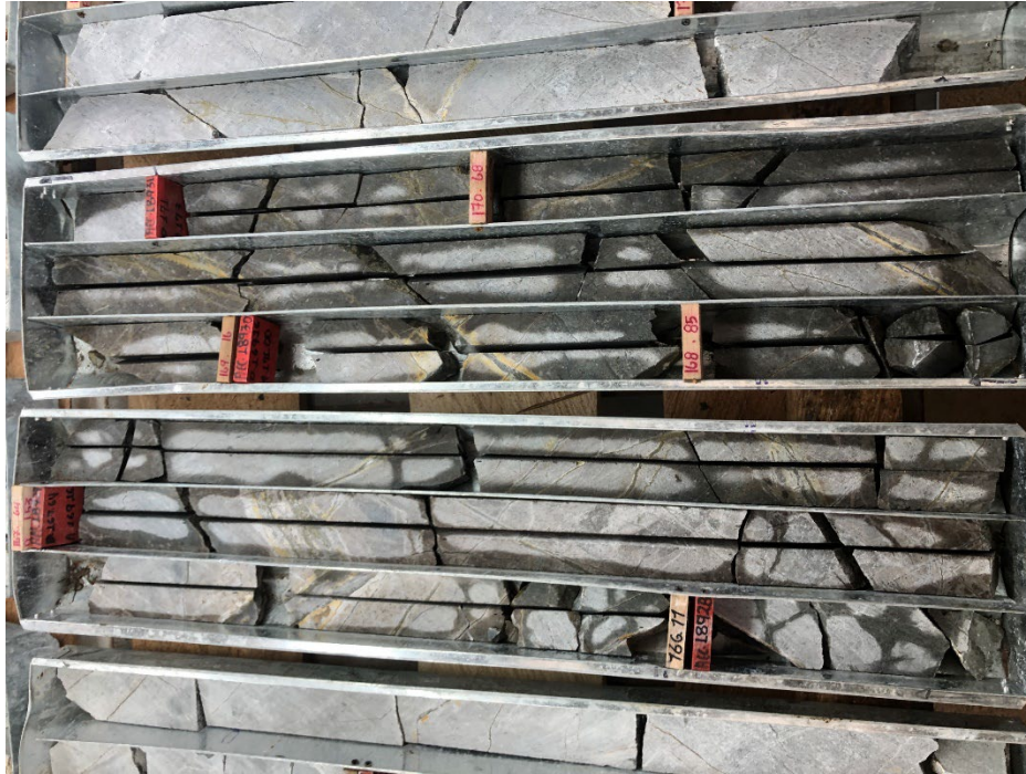
Figure 12-13 ¼-core for duplicate checks ready for sampling as prepared under the supervision of the QP during the current site visit
