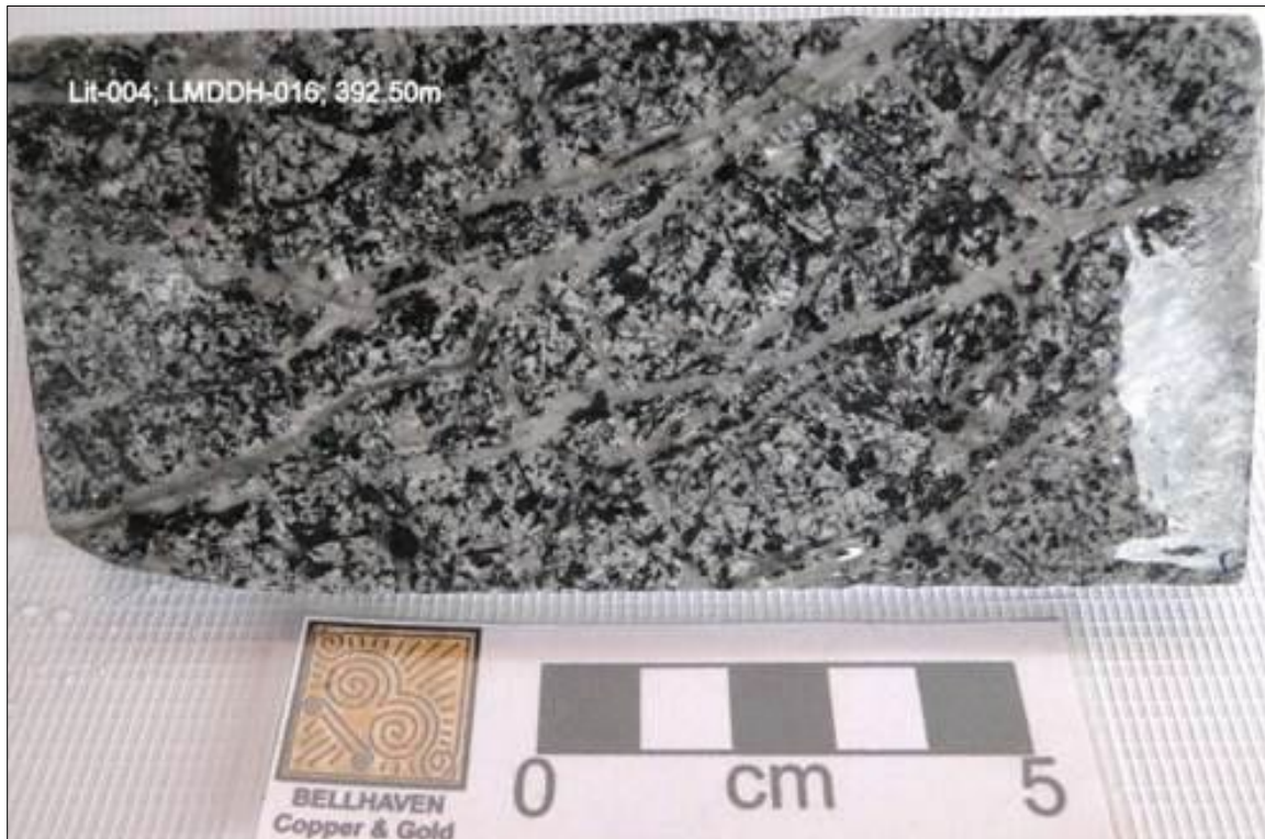
Figure 7-7 LMDDH-016 392.5m. C1 Breccia with Potassic Alteration (Magnetite-k-Feldspar +/- Actinolite) Cut by Sheeted Magnetite Veins, Quartz Magnetite Stockwork Veins and Late Pyrite-filled Fractures
